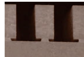
Cross section showing Reactive Ion Etching and Cross section of RIE etching (Courtesy of MEMSCAP)
